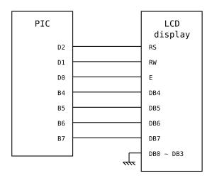
Supply the PIC and the LCD display with 5V.
